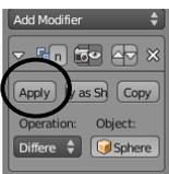
By hitting the “**Apply**” button, the new shape becomes set and the sphere can be removed.
