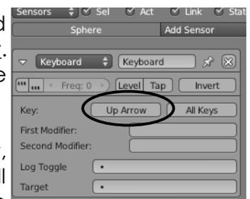
Think of the *Controller* as the computer processor. By default, we hit "And", meaning that if we tie more than 1 sensor to it, all sensors must be in a true state in order for an actuator to function. There are other expressions available in the controller.
