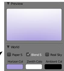
When setting just a straight gradient color for your world, Select the "Blend" option above the color swatches and set the Horizon and Zenith colors.
