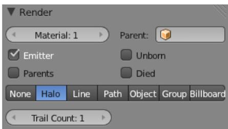
The **Render** panel provides setting for what the particles look like rendered (F12) or animated. If the *Emitter* button is not checked, you will see the particles and not the mesh that they are emitted from. You can also chose to see *Unborn/Died* particles. Particles can also be represented different ways such has *Halo* (material settings), *Line*, *Group*, or an actual *Mesh* Object.
