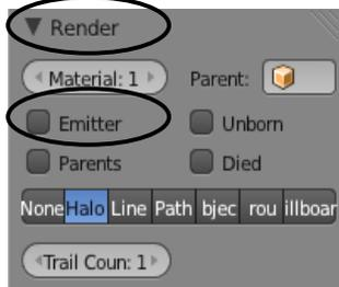
You may see the actual sphere in the center of the explosion. To turn this off, go to the Render panel under particles (if you had the camera selected from before, select the sphere again) and turn off "Emitter" so the actual mesh doesn't render. You could also experiment with Trail Counts for a second release. To improve the explosion, add a material and adjust the Halo setting. (review chapter 4) Adjust the Diffuse Color, Halo Size and try Lines and Stars. You should end up with a nice effect.
