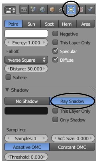
To get a ray shadow for a lamp, select the lamp you want to cast shadows (all types work with ray-tracing), go to the **Lamp** settings, find the "Ray Shadow" button and activate it.
