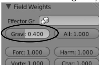
downward a bit to much, so we'll fix that next. Go down to the *Field Weights* panel and set *Gravity* to about 0.40. Feel free to experiment with these setting for different effects.
